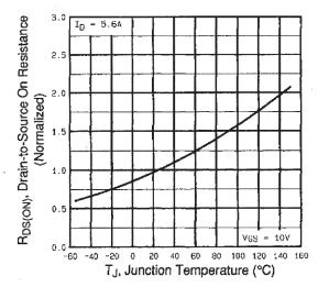
Fig. 4 - Normalized On-Resistance vs. Temperature
