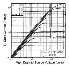
Fig. 2 - Typical Output Characteristics,  $T_C = 150$  °C
