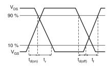
Fig. 10b - Switching Time Waveforms
