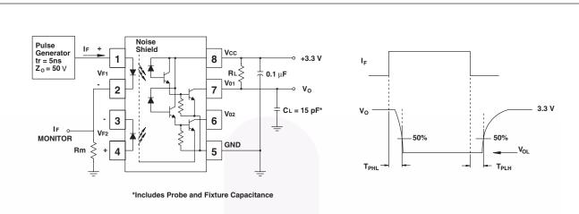
Fig. 9 Switching Time Test Circuit
