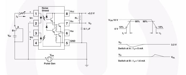
Fig. 10 Common Mode Immunity Test Circuit
