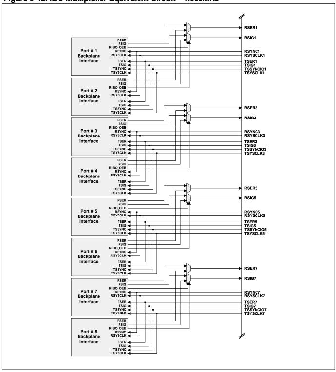
Figure 9-12. IBO Multiplexer Equivalent Circuit—4.096MHz
