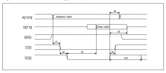
Figure 13-3. Intel Bus Write Timing (BTS = 0)
