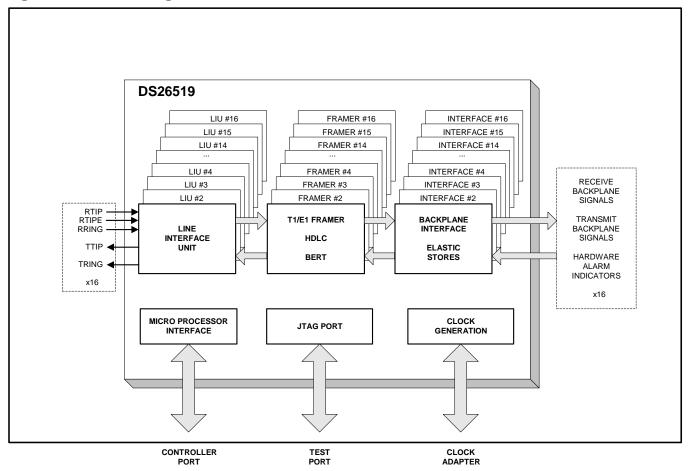
Figure 7-2. Detailed Block Diagram
