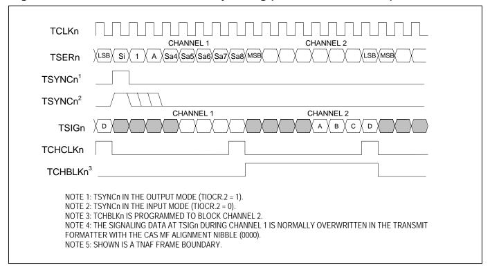
Figure 11-26. E1 Transmit-Side 1.544MHz Boundary Timing (Elastic Store Enabled)
