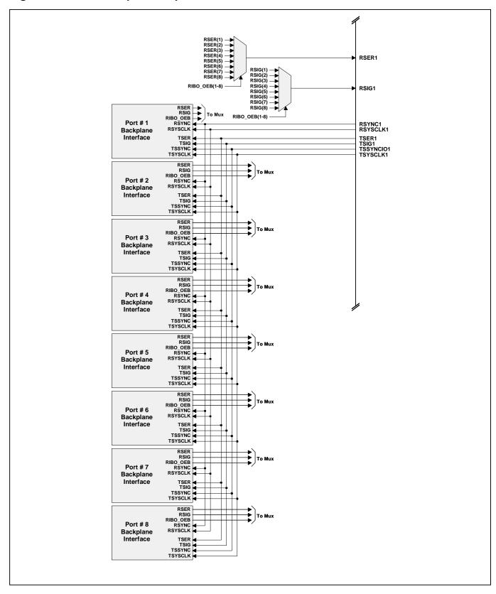
Figure 9-14. IBO Multiplexer Equivalent Circuit—16.384MHz
