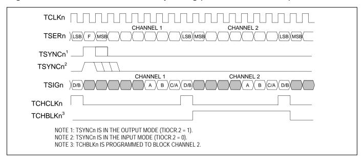
Figure 11-12. T1 Transmit-Side 1.544MHz Boundary Timing (Elastic Store Enabled)
