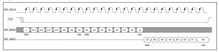
Figure 9-2. SPI Serial Port Access for Read Mode, SPI\_CPOL = 1, SPI\_CPHA = 0
