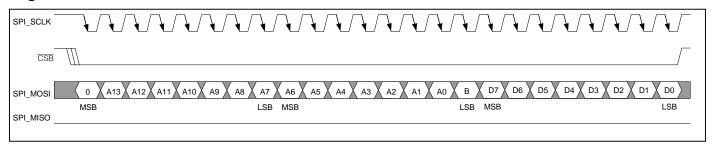
Figure 9-7. SPI Serial Port Access for Write Mode, SPI\_CPOL = 0, SPI\_CPHA = 1
