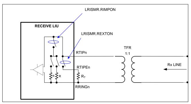
The device couples to the receive E1 or T1 twisted pair (or coaxial cable in  $75\Omega$  E1 applications) via a 1:1 or 2:1 transformer. See <u>Table 9-40</u> for transformer details.
