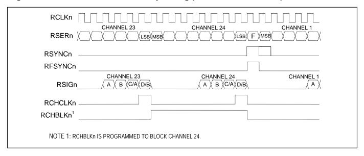
Figure 11-4. T1 Receive-Side 1.544MHz Boundary Timing (Elastic Store Enabled)
