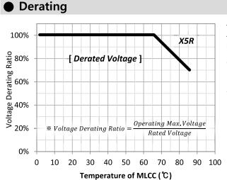
This product ,which guarantees High Temperature Reliability Test with 100% of rated voltage at the maximum temperature, recommended to be used in the circuit with derat is recommended to be used in the circuit with derated voltage compared to the rated voltage of the capacitor for long lifetime.
