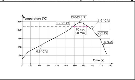
Figure 22. ST ECOPACK<sup>®</sup> recommended soldering reflow profile for PCB mounting
