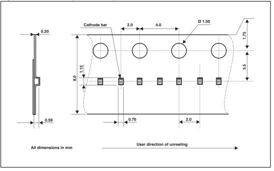
Figure 19. SOD882 tape and reel specifications
