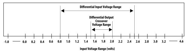
Figure 12. Differential Receiver Input Sensitivity vs. Common Mode Input Range
