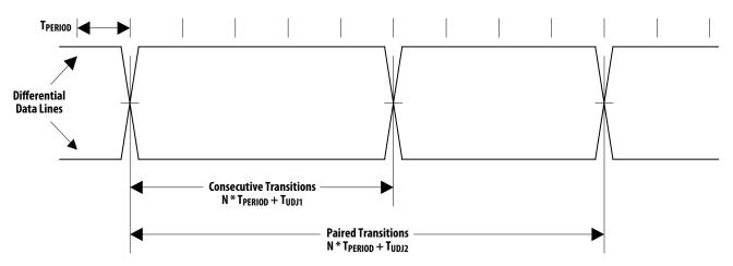
Figure 15. Differential Output Jitter
