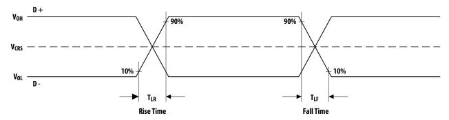
Figure 10. Data Signal Rise and Fall Times
