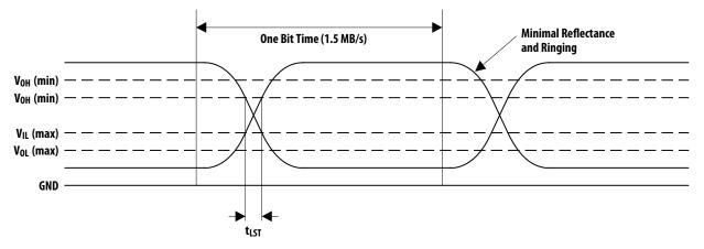
Figure 11. Data Signal Voltage Levels
