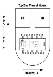
Figure 1c. Package pinout at 270°
