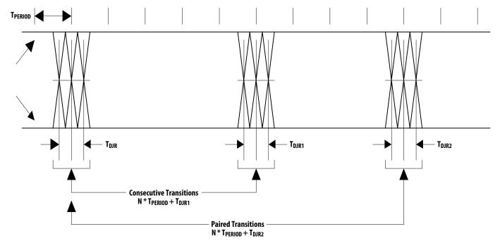
Figure 13. Receiver Jitter Tolerance
