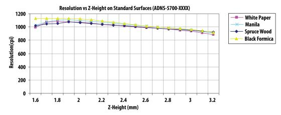
Figure 16. Typical Resolution vs. Z Height
