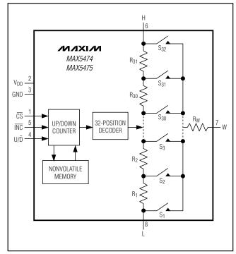
Figure 3. MAX5474/MAX5475 Functional Diagram
