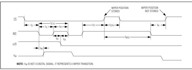
Figure 1. Digital Interface and Timing Diagram
