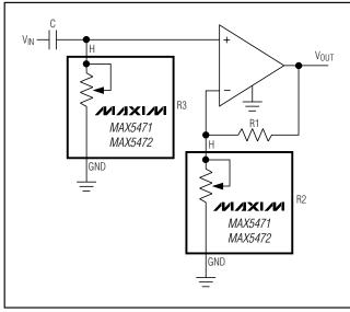
Figure 6. Programmable Filter
