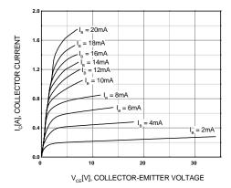
Figure 1. Static Characteristic
