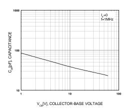
Figure 4. Collector Output Capacitance
