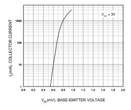
Figure 5. Base-Emitter On Voltage
